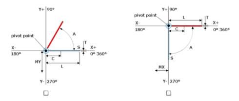
The gas spring must not be exposed to any possible side or twisting forces due to misalignment of the assembly, it will cause friction to the seals and consequently prematurely failure. A gas spring should be able to pivot freely in its brackets if not, premature failure or bending will occur.
